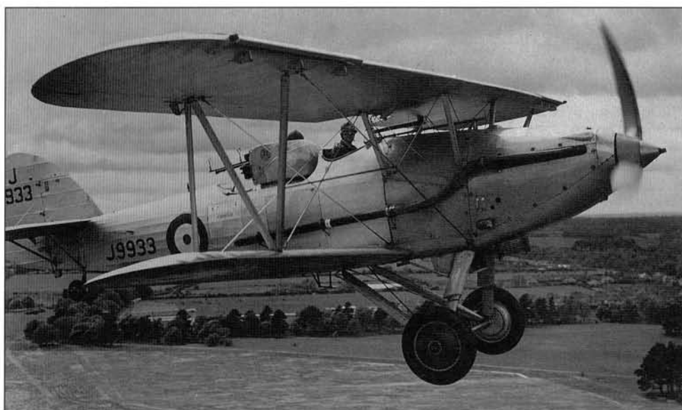
Left This photograph shows the prototype Demon, built as a Hart bomber in 1929, taking off from Brooklands featuring the Frazer-Nash 'lobster-shell' turret, fitted in May 1934
