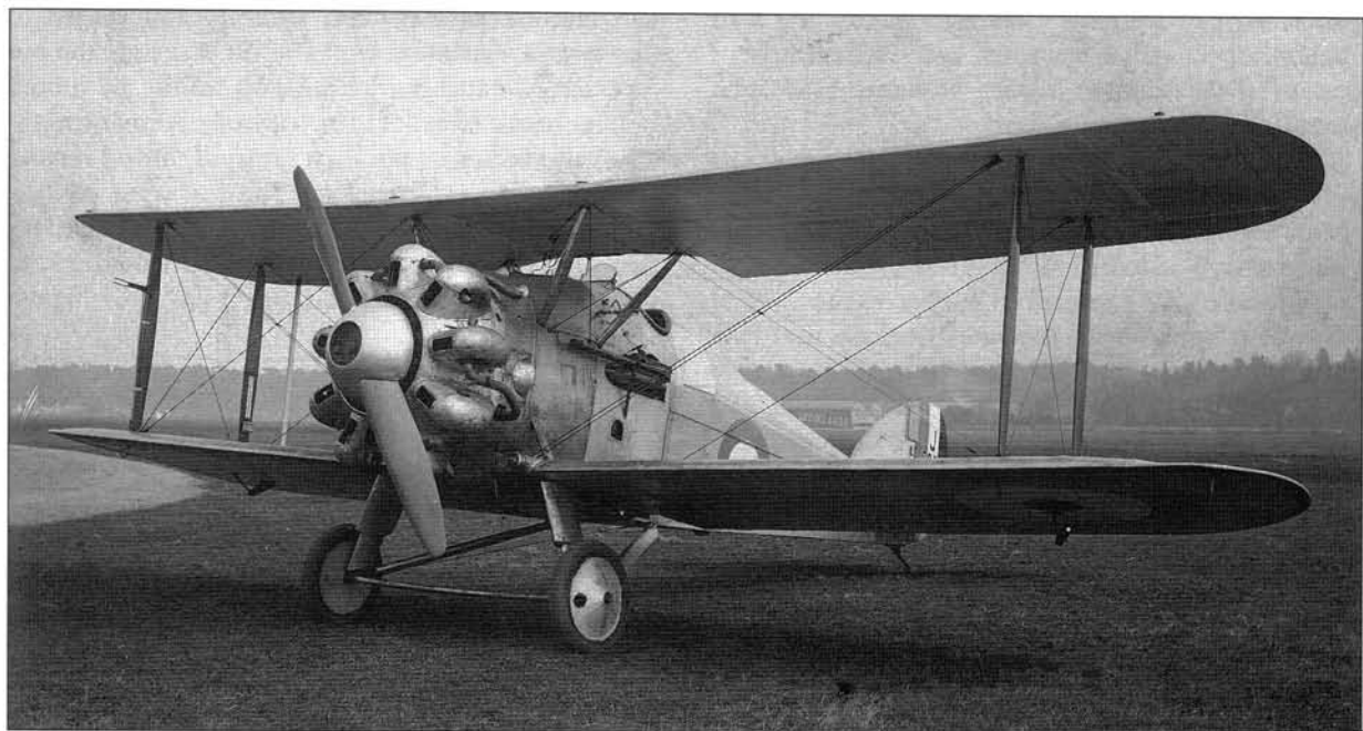
Above The cowled Bristol Jupiter Mk IV radial engine of the second Woodcock prototype, J6988
