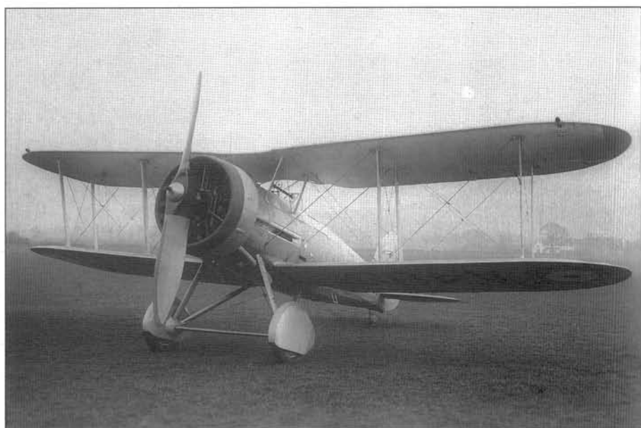
Above J9125, now the SS.19B, fitted with Mercury VIS2 and sporting a tailwheel, flying in April 1934
