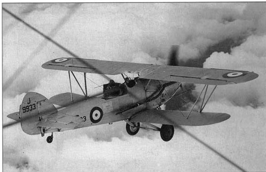
Left Another view of the Demon prototype fitted with the Frazer-Nash turret. J9933 eventually became an instructional airframe in August 1938
