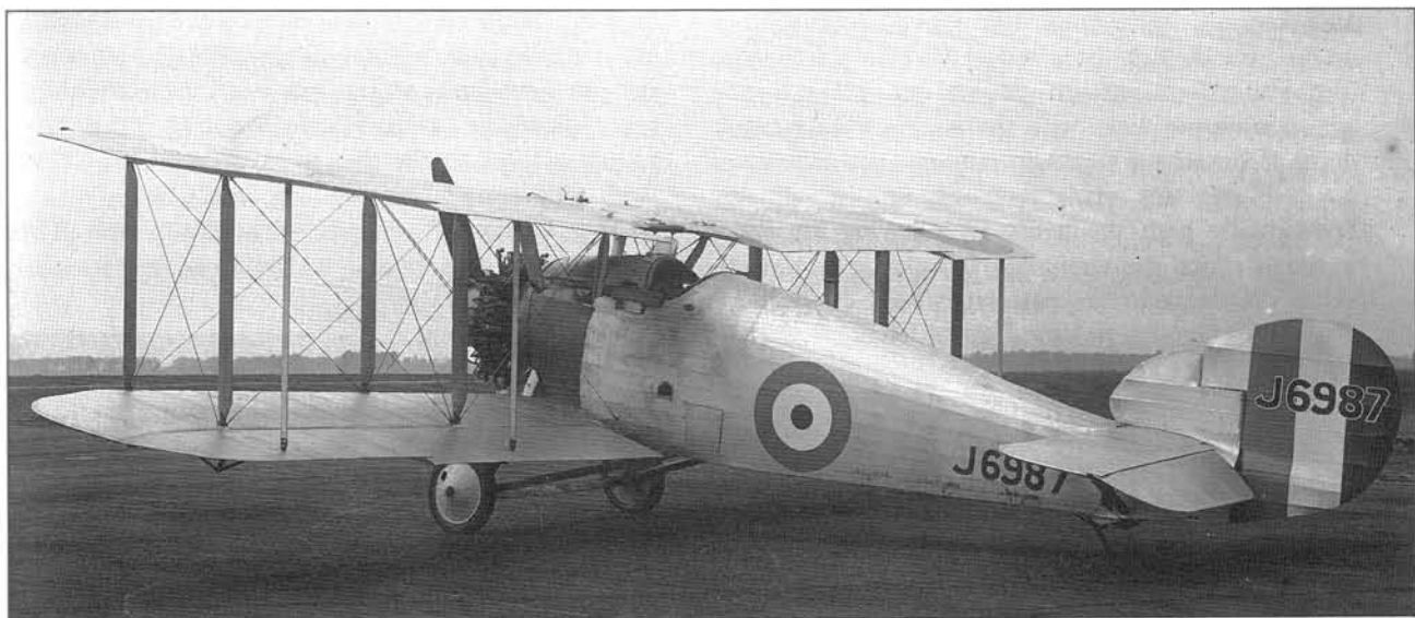
Above A photograph of the first prototype Hawker Woodcock J6987, fitted with its third fin and rudder. Note too the addition of tailplane struts – the elevator controls were now within the fuselage
