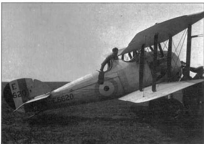
Left Two-seat Snipe E6620. Although used mainly at FTSSs, one or two of these dual-control trainers were issued to most of the Snipe fighter squadrons. This simple conversion was carried out at Sopwith's Kingston-upon-Thames factory
