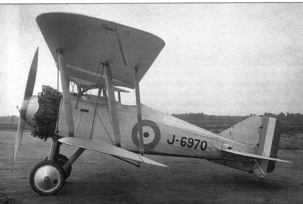
Left Gloster's second prototype Grebe was J6970, which, like J6969, boasted fairings for the type's twin .303in machine guns. These covers were later dispensed with prior to the aircraft entering squadron service
