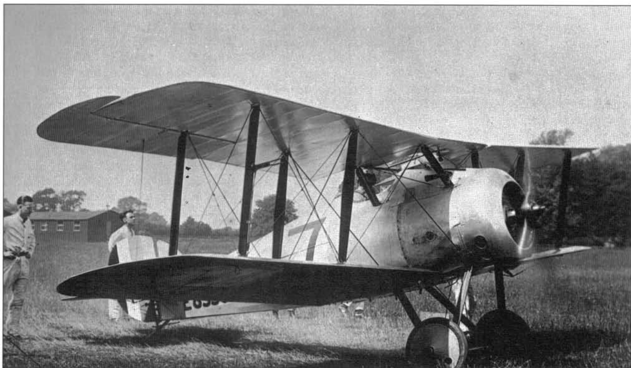
Above Flattening out the grass with his prop wash, a student pilot carefully runs his mount's Bentley B.R.2 engine up to full revs prior to taxiing out for take-off
