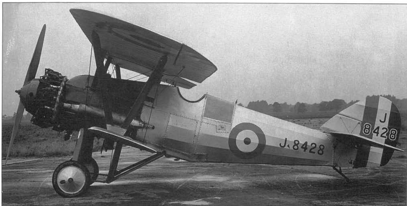
Above J8428 fitted with heater muff on the engine exhaust. First flown in October 1925, this Siskin spent much of its life to-ing and fro-ing between the RAE and its makers
