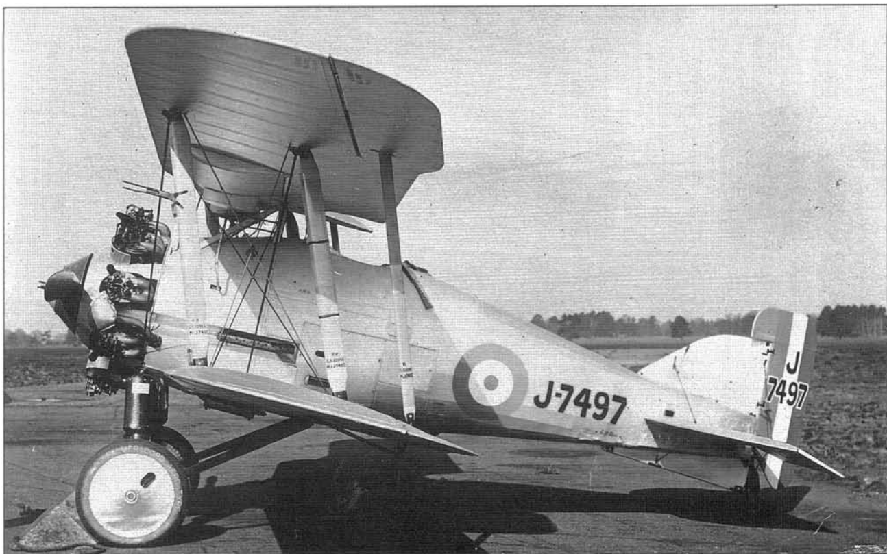
Above The first prototype Gamecock, J7497, after installation of a horn-balanced rudder
